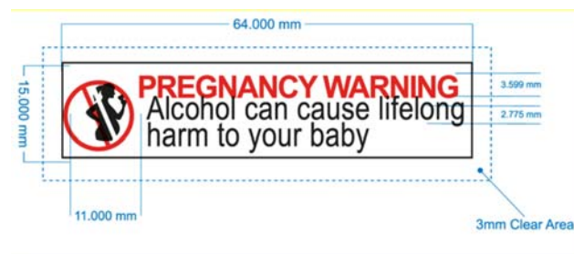
Figure 2: Example of a misaligned pictogram within the pregnancy warning mark
